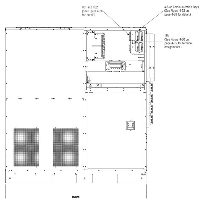
Figure 4-27. ISBM Section Interface Terminal Locations
